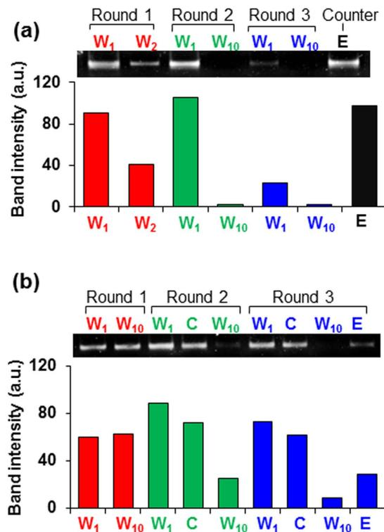
**Figure 4.** Gel electropherograms showing progress in the isolation of target-binding aptamer candidates during multi-round microfluidic SELEX. Bar graphs depict the band intensity in the gel images from eluents collected during the SELEX process for (a) IgE and (b) BA-glucose mixture. Lane W: wash; Lane C: counter selection; Lane E: elution.
