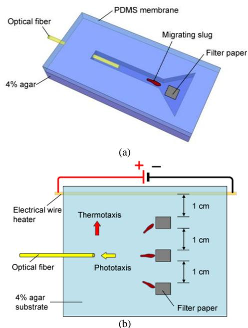
Figure 2. Schematics of agar microchips used for (a) slug phototaxis in a microchannel and (b) simultaneous phototaxis and thermotaxis on an agar substrate.
