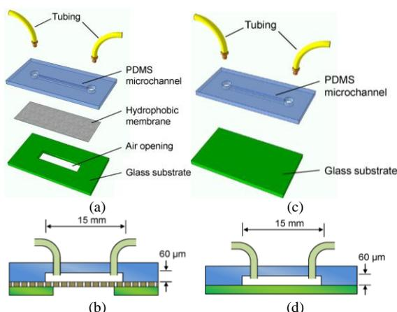
Figure 1. (a) Design schematic and (b) cross-section view of a microchip with an air perfusion component. (c) Design schematic and (d) cross-section view of the chip lacking an air perfusion component.
